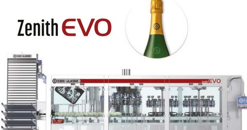
Feeding, dispensing and application of sparkling wines capsules with double centring system: orientation of the bottle (embossed logo on glass, screen print, sleeve and glass mould seaming) and capsule, both with cameras managed by SNIPER vision system.
