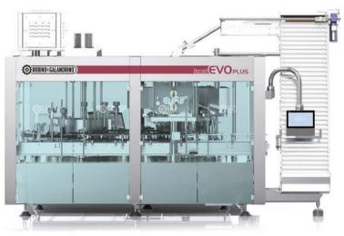
Wirehooder featuring bottle orientation (embossed logo on glass or glass mould seaming) prior the application of wirehoods achieving the desired position of the opening eyelet (via SNIPER vision system).
